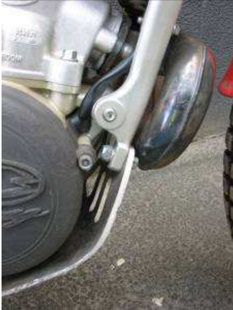
Figure 9 Bumper fastening bolt
